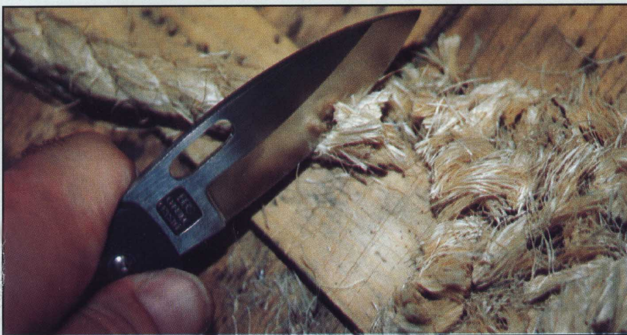
Fifty-seven cuts on the half-inch sisal rope puts the Boye piece in the author's upper echelon of aggressive-cutting knives.
