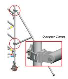
Immediately below the Platform/Handrail/Midrail level only one yellow coded Diagonal Bracing per side is needed. They should slope in opposite directions.
