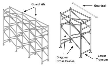
When H Frames are set up as a multi-bay scaffold EASY ACCESS GUARDRAIL POSTS must be used to support guardrails and cross bracing mid-rails as shown.
