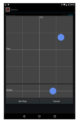
Set the start and end points for the SMS mode. This can also be used for video shots. Port 1 is Pan, Port 2 is Tilt, and Port 3 is Slide.
