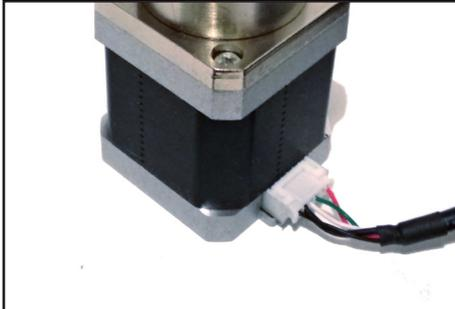
2. Plug the motor cable into the motor.
