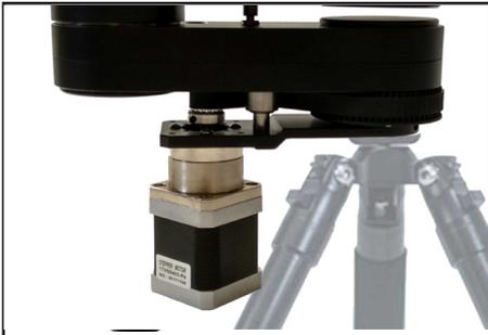
1. Hold the motor **NOT** the Wing Arm when attaching tripod legs
