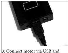
3. Connect motor via USB and power to the controller.
