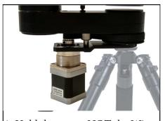
Hold the motor **NOT** the Wing Arm when attaching tripod legs
