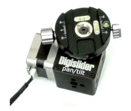
There are two locks on the panning head. The larger one is to lock the arca swiss plate, the smaller is to lock the panning unit. Clockwise to tighten. Make sure it is tightened when the motors are moving.
