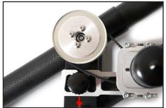
4. Pull down to attain tension and fasten tight to secure.
