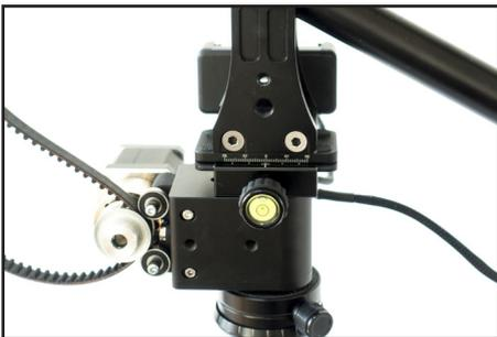
5. Attach the Pan Tilt System to the jib.
