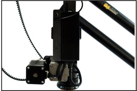
10. Add the Controller and the battery to the side of jib.
