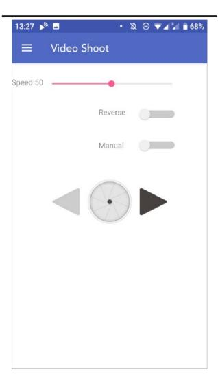
Select the speed of the video. Slide the bar next to "Reverse" to turn on or off continuous loop mode (Default is off). Press the centre icon to start the video. The arrows will allow you to change direction in real time. You can also change the speed in real-time.
