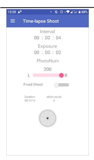
Set the Interval/Frames (Time between each shot/frame). Set Exposure/Shutter (Exposure time available). If your camera is in Bulb mode the app will trigger the camera's shutter for this amount of time. Set the number of photos. The duration will change below. Press the icon to start.
