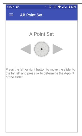
Enter "AB Point Set" from the main menu screen and set the start and end points. Press the left or right arrows to move in that direction and the centre icon to set A which is the start. Do the same again for B which is the end position.
