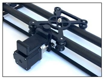
Loosen the thumb screw on the carriage and slip the motor with belt attached into the slot and tighten to secure it in place.
