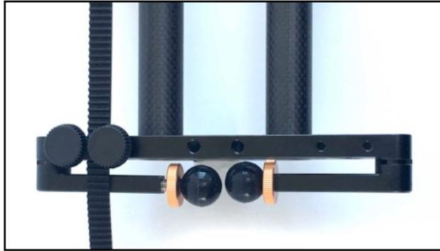
Use the thumb screws underneath to attach the belt.
