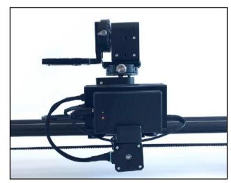
Attach cables and battery or battery holder. Mount the controller and power in the attached spring loaded clamp on top of the motor.
