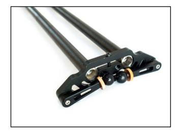
The rods fit into the ends of the slider feet and secure with the bolt in the top. Use the allen key hex set to tighten and secure the rods. Only do this to one end first.
