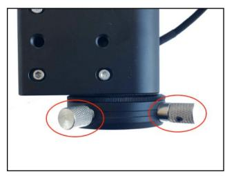
This bottom plate of the pan unit should be attached to the carriage. The thumb screw of the left loosens the plate. The thumb screw on the right can be pulled to release/secure the plate.
