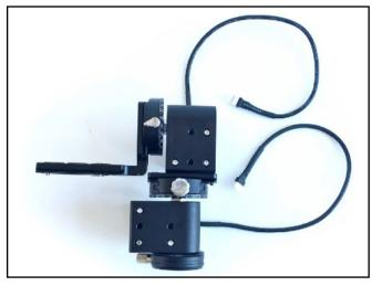
If you have purchased a 2nd rotary unit for the Tilt axis, attach both together with the L-bracket.
