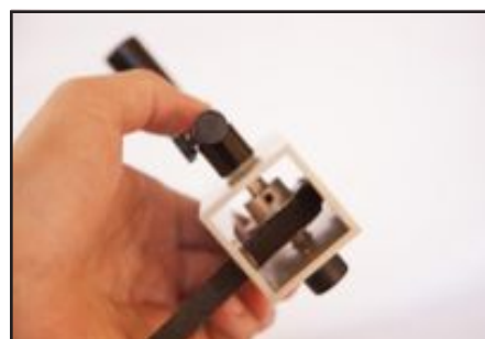
44. Push through with finger (rotating the pulley if needed)...
