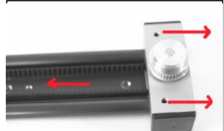
63. ...one is pulled away from the end. Cut belt shorter if required*
