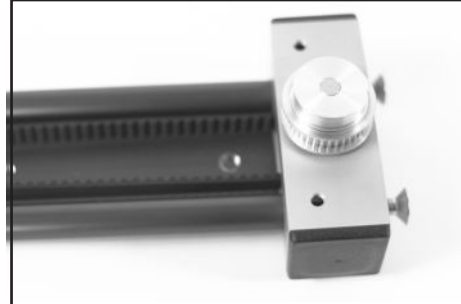
65. Place Box over end so there are no gaps. Then screw (16.) into...
