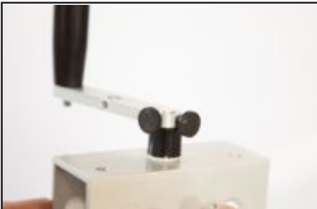
34. Insert last Thumb Screw (9.) into end.
