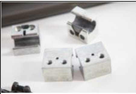
61. Slide the 4 Carriage Blocks onto rail, 2 each side.
