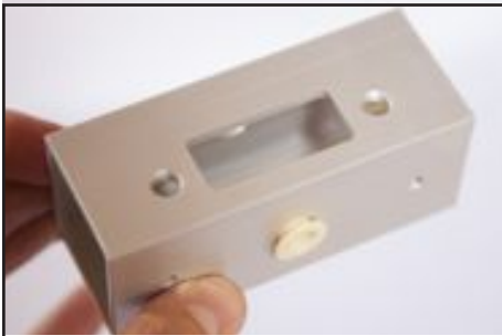
19. Insert 3rd Shaft Bearing (3.) into bottom of 2nd Pulley Box (2.).
