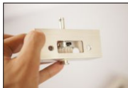
14. Insert Long Grub Screw (7.) and tighten with Allen Key (22.).
