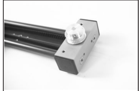
66...holes, alternate every 1cm until tight with Allen Key.
