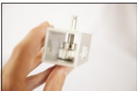
13. Align both pulley holes over both Shaft (4.) holes.
