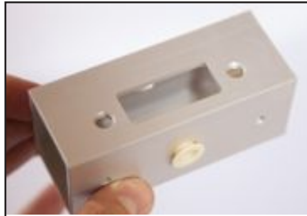
2. Insert 1st Shaft Bearing (3.) into Pulley Box (1.).
