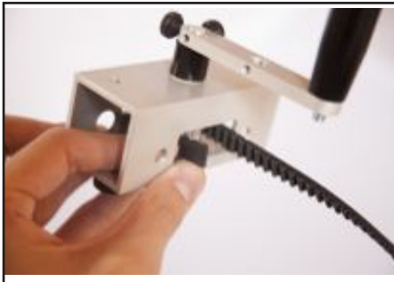
47. ...and rotate so the end comes through.
