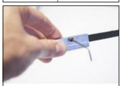
52. Place the Outer Belt Clip (18) over and secure with...
