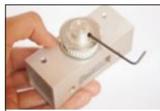
18. Rotate Shaft and insert Short Grub Screw (8.) and tighten.
