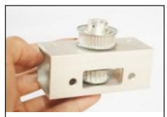
16. Insert Large Pulley (6.) over Shaft and align both holes.
