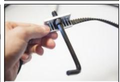
54. Insert the Large Belt Screw (20.) through both.
