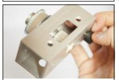
37. Screw into bottom of Pulley Box.
