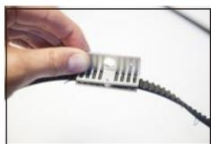
51. Place the belts teeth into the slots of the Inner Belt Clip (19).
