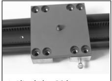
70. Align holes. Make sure resistance screw is loose.
