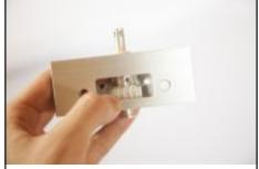
12. Insert Shaft (4.) through bottom hole.
