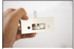
15. Rotate Shaft and insert Short Grub Screw (8.) and tighten.
