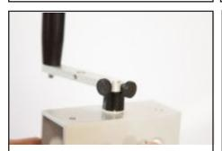
34. Insert last Thumb Screw (9.) into end.
