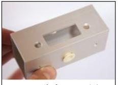
2. Insert 1st Shaft Bearing (3.) into Pulley Box (1.).
