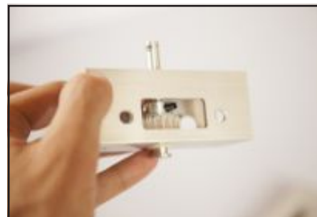
29. Insert 2nd Long Grub Screw (7.) and tighten with Allen Key
