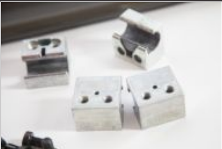
64. Slide the 4 Carriage Blocks onto rail, 2 each side.
