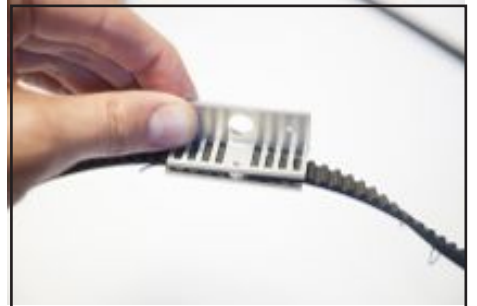
51. Place the belts teeth into the slots of the Inner Belt Clip (19).
