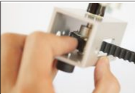
46. Push the end of the belt against the pulley...
