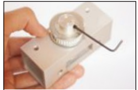
18. Rotate Shaft and insert Short Grub Screw (8.) and tighten.
