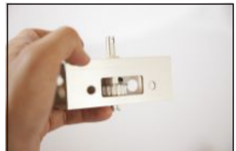
30. Rotate Shaft and insert 2nd Short Grub Screw (8.) and tighten.
