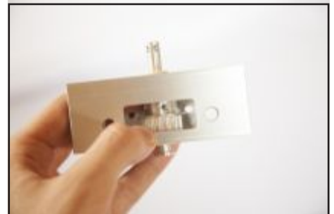
27. Insert last Shaft (4.) through bottom hole.
