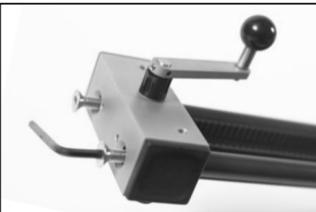
67. Place second Pulley over other end of rail and screw in.
