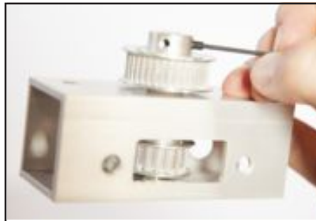
17. Insert Long Grub Screw (7.) and tighten with Allen Key (22.).
