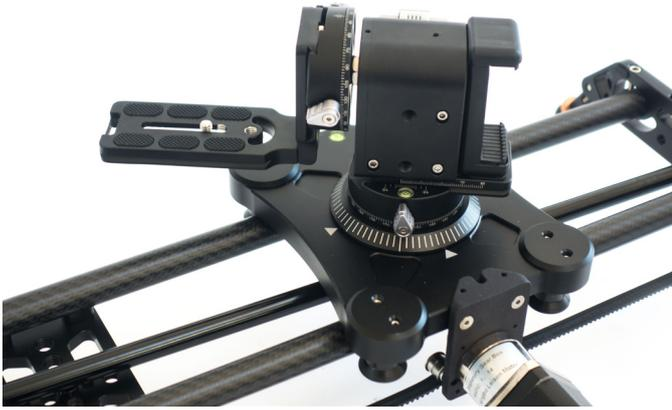
The Tilt kit can be mounted onto the carriage by screwing into place. There are 2 silver pins in the side, one pulls out to allow quick removal or insertion of the base which will need to be fastened to the carriage. The second fastens and locks the tilt kit in the position you desire.
