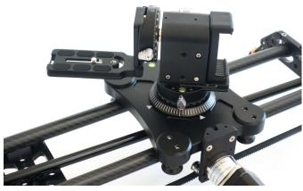
The Tilt kit can be mounted onto the carriage by screwing into place. There are 2 silver pins in the side, one pulls out to allow quick removal or insertion of the base which will need to be fastened to the carriage. The second fastens and locks the tilt kit in the position you desire.
