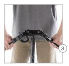
**Expand** the handlebars until the handlebar sleeves click into place. (Be careful not to wrap the handlebar wires around the dashboard unit.)
