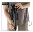
Loosen the T-bar tightening knob.
