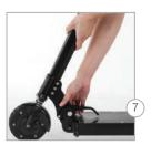
**Lift** the stem, so that the front wheel is slightly off the ground, then **press down** the fixing lever.
