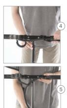
Loosen the T-bar tightening knob.
