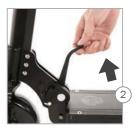
Lift up the securing lever and secure it against the stem.
