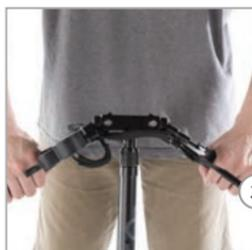
**Expand** the handlebars until the handlebar sleeves click into place. (Be careful not to wrap the handlebar wires around the dashboard unit.)
