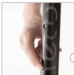
5 **Push in** the positioning pin and **push** the T-bar extension down into the stem.
