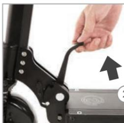
**Lift up** the securing lever and secure it against the stem.
