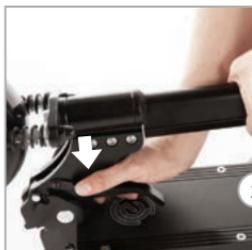
**Press down** the fixing lever, and lift up the stem from the deck until it clicks into place.
