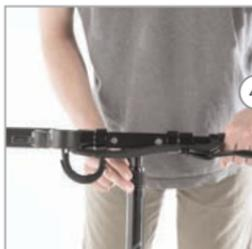
4 **Loosen** the T-bar tightening knob.
