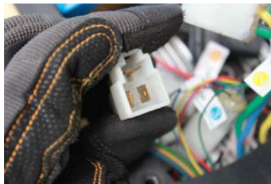
A3. Unplug the connector with '2. motor' and '3. hall sensor', then try to check if there is anything bended. Adjusted them if needed or bend it a bit to create a better contact.
