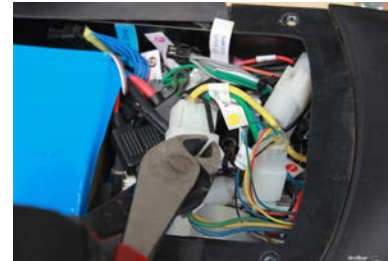
A2. Find out the connector with label '2. motor' and '3. hall sensor', then cut off their cable tights.
