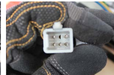
A3. Unplug the connector with '2. motor' and '3. hall sensor', then try to check if there is anything bended. Adjusted them if needed or bend it a bit to create a better contact.
