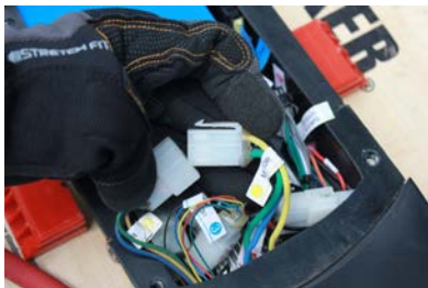
A3. Unplug the connector with '2. motor' and '3. hall sensor', then try to check if there is anything bended. Adjusted them if needed or bend it a bit to create a better contact.
