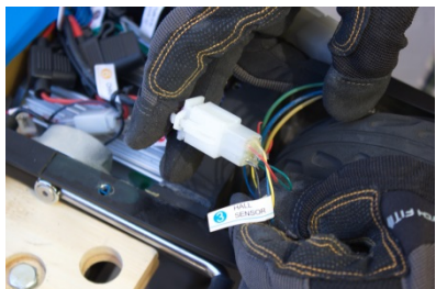
A4. Remove the hall sensor and motor connection.
