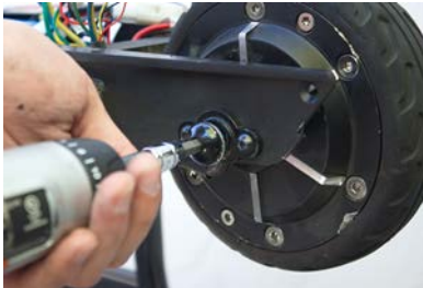
B2. Lock the wheel and put the rear fender back.
