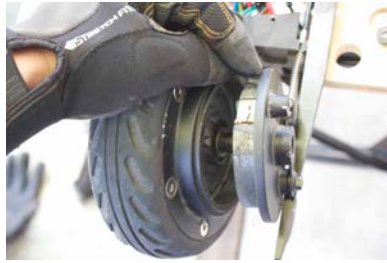
B1. Put together the wheel and brake plate, insert it back to the scooter.
