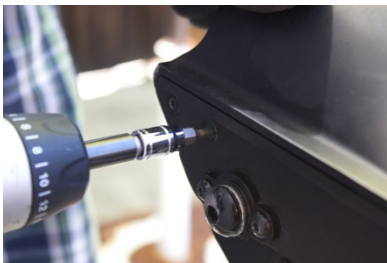
B4. Screw the rear fender back on, then to put the rubber piece back on top.
