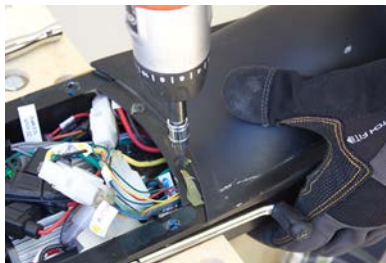
B4. Screw the rear fender back on, then to put the rubber piece back on top.
