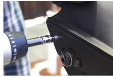
A3. Remove the foot desk and use a heat gun to melt the thread-locking glue on the screws. Then take off the rear fender. (There are 5 screws to lock the rear fender. The front of two screws are using H2.5 and the others is using H3 hex driver)
