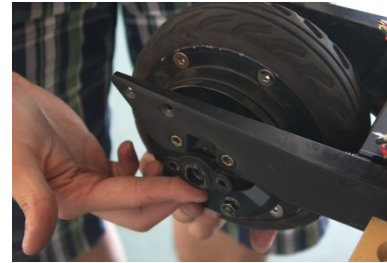
B1. Put together the wheel and brake plate, insert it back to the scooter.
