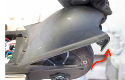
A3. Remove the foot desk and use a heat gun to melt the thread-locking glue on the screws. Then take off the rear fender. (There are 5 screws to lock the rear fender. The front of two screws are using H2.5 and the others is using H3 hex driver)
