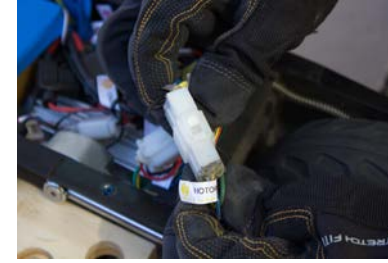
B3. Connect the hall sensor and motor connectors.
