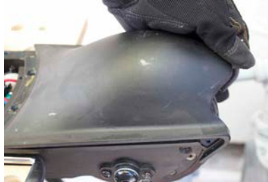
B2. Lock the wheel and put the rear fender back.
