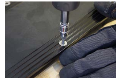
B5. Screw the foot deck on. Installation is done.
