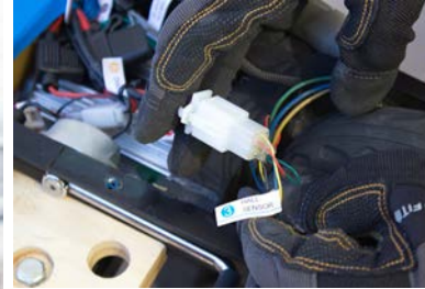
B3. Connect the hall sensor and motor connectors.
