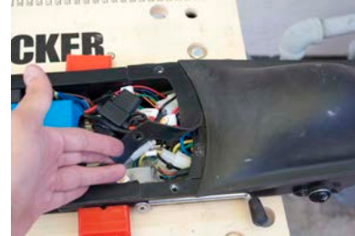
A2. Take off the rubber piece to expose and release the screws.
