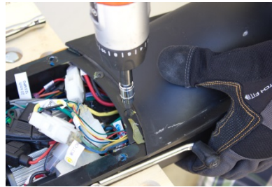
A3. Remove the foot desk and use a heat gun to melt the thread-locking glue on the screws. Then take off the rear fender. (There are 5 screws to lock the rear fender. The front of two screws are using H2.5 and the others is using H3 hex driver)
