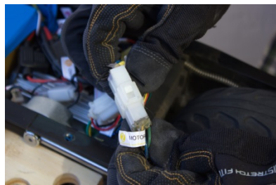
A4. Remove the hall sensor and motor connection.
