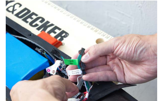
2. Identify 3 pairs of connectors with matching colors (labeled kick-start, 12.5 mph, and 7.5 mph) near the rear wheel wire.
