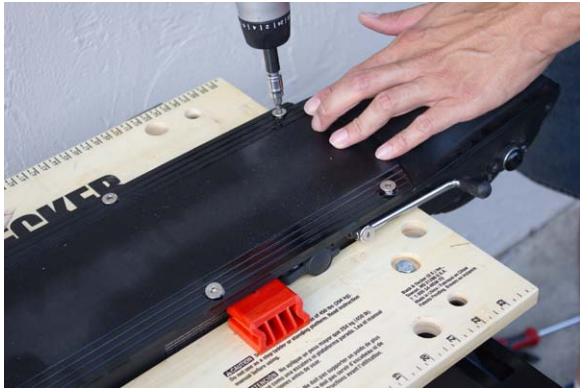
1. Open the foot deck using a hex driver (8 screws).
