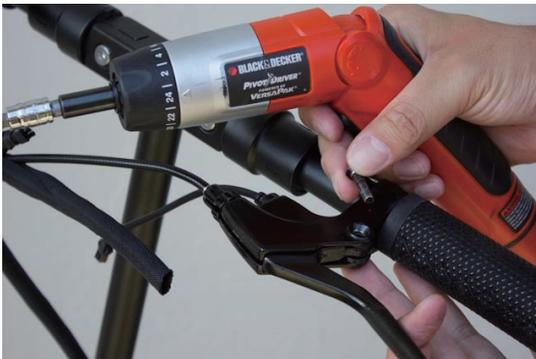
B2. Unscrew and remove the hex screw that hold the brake lever together on the holder
