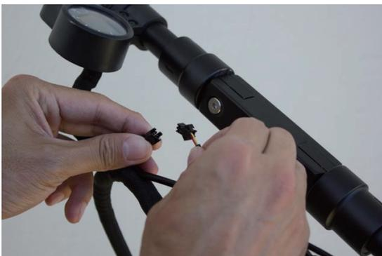
A3. After you disconnect the brake signal wire, please check the wiring near the connector of the brake end (in the right hand in the image).
