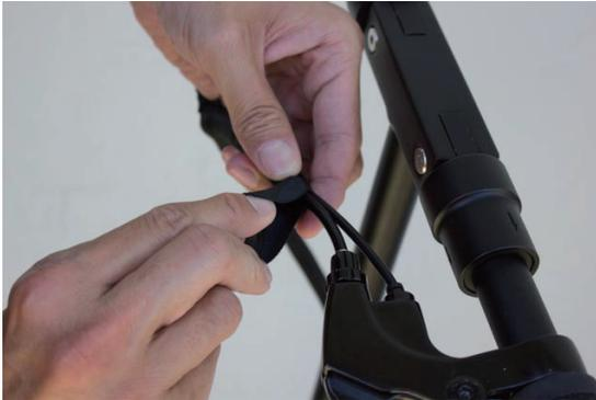
A1. Unwrap the cable wrap near the brake wire
