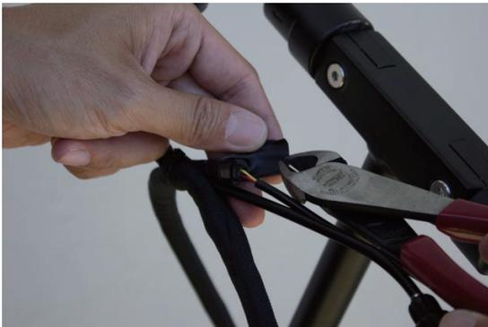
A2. Remove the heat shrink tube to access the connectors
