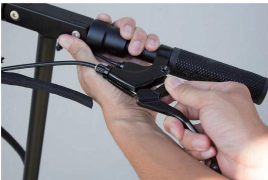
B3. Put the screw, small spring, and 2 plastic reducers down
