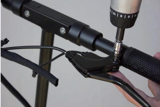
B1. To check that, you would need to remove the brake lever by untightening the screw
