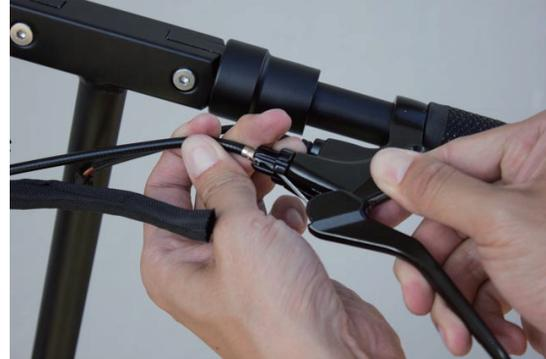
B4. Pull the brake lever away from the brake lever holder and make the brake pull wire go thru the side gap
