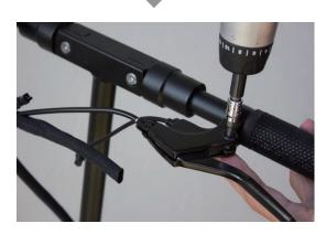
B1. To check that, you would need to remove the brake lever by untightening the screw
