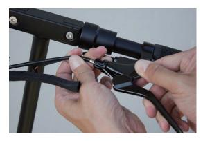
B4. Pull the brake lever away from the brake lever holder and make the brake pull wire go thru the side gap
