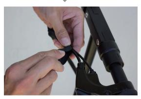
A1. Unwrap the cable wrap near the brake wire
