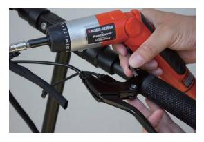
B2. Unscrew and remove the hex screw that hold the brake lever together on the holder
