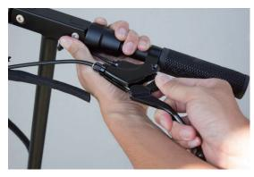
B3. Put the screw, small spring, and 2 plastic reducers down
