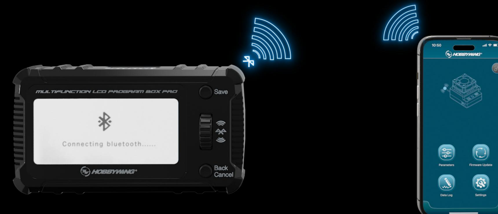
The built-in Bluetooth module functions as an OTA **Programmer.** The ESC establishes a wireless connection with a smartphone through the LCD programming box.
