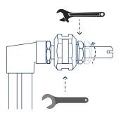
**3.** Use the Multi-Fuel Adapter Installation Wrench to hold the adapter and prevent it from spinning. Tighten the Tip Nut. DO NOT OVERTIGHTEN.
