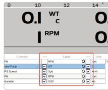
In the page showing the RPM bar graph you can set the channels you prefer in any field. Please note that lap times – i.e. Best, Predictive, Rolling, +/- Best – are to be shown on the right fields only. Hiding channel label, the lap time visualization becomes bigger.
