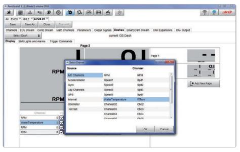
Once all the channels have been set, you can enable/disable or modify each channel label and show/hide its measure unit.
