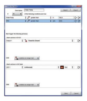
Describe the Alarm: it can be a single event like "Water temperature higher than 100°C" or a combination of events, like in the example: "Water temperatures higher than 100°C" and "RPM is higher than 6000". Describe what to do when an alarm arises.
