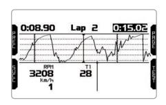
If you just finish the test the first page you see is the one here on the right. The page shows the three best laps of that test with max/min RPM values and RPM drop.
