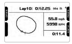
This page shows the lap sectors with max/min speed and related RPM values.
