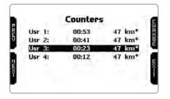
Each odometer can be activated/deactivated and/or reset. Select the odometer you want to manage and press "CHANGE":
