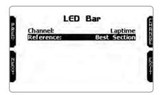
Choosing "RPM" (left image below) you can set RPM threshold value (up to 16.000) that switches on each LED so to know when shifting. Choosing "OFF" the central LED bar is disabled.
