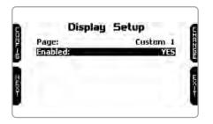
Each custom page can show up to four fields. Pressing "SELECT" you can choose the channel to show in each field. The only field that can show lap time in different formats is bottom right one (right image below).
