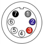
7 pins Binder 712 male connector pinout solder termination view
