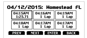
"Lap Summary" is to be enabled as explained in paragraph 5.1. This page shows the three best lap of the test with max speed value per every lap.
