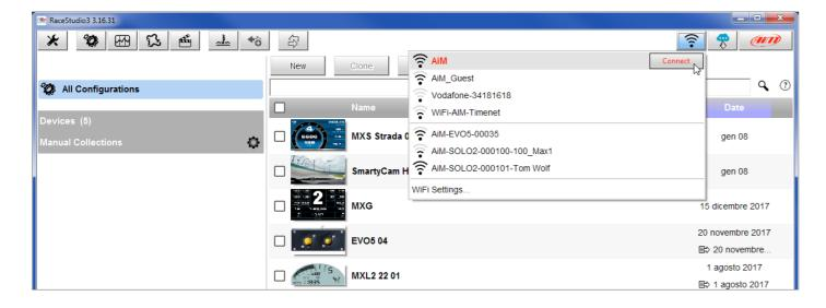
When the PC is authenticated to the network called "AiM" it can see all devices you configured to access the same network. In the image below two AiM devices are connected to the same "AiM" WLAN.
