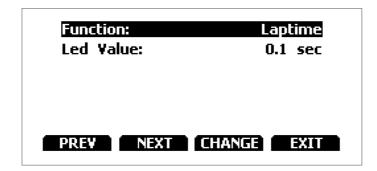
Here you can set the 10 lateral LEDs of Solo 2 function and working mode (value). Function can be:
