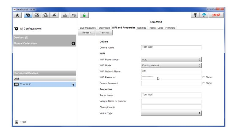
Here above you see a device "Solo2-00101" that switched from AP to WLAN mode (Existing Network). Network name is "AiM" and does not work with free access because is protected by a password. To obtain connectivity on the device the PC has to be authenticated to the same network as shown here below.
