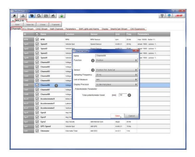
When the software comes back to "Channels" layer the potentiometer has been set on the desired channel as shown here below.
