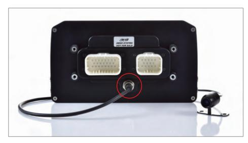
Rear cameras needs to be connected to the logger, set in the logger configuration through Race Studio 3 software and executed through the logger keyboard. Here follows explanation of how to perform all these operations.
