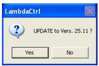
• if the firmware version offered (in the figure the system offers firmware version 25.10) is more recent that the one installed on **LCU-ONE Analog** (supposing the one installed is version 25.08), press "Yes" and upgrade the controller firmware
