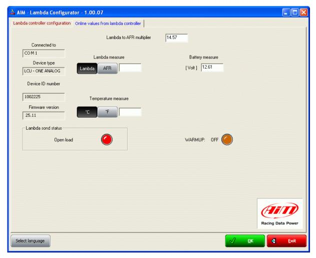
This panel shows controller status. The user is only allowed to set Lambda/AFR and temperature unit of measure for the values shown in this panel.
