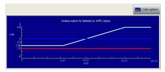
The "analog output graph" shows output tension values of the controller in correspondence of the measured Lambda values. Graph colours are customizable. Pressing "Colour options" button the window shown below appears:
