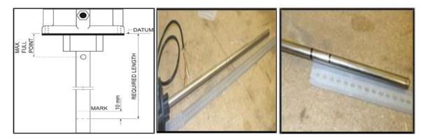
When cutting the metal shaft can be lightly gripped in a soft jaw vice but do not crush the outer shaft as this would render the sender unusable. The outer shaft can be cut with a pipe cutter. Don't advance the cutter too quickly as this could deform the outer shaft.
