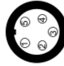
5 pins Binder 712 female connector pinout solder termination view
