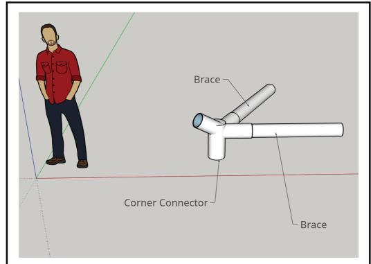
INSERT 2 BRACING TUBES INTO INWARD FACING SOCKETS OF THE CORNER CONNECTORS
