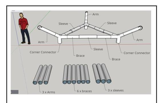
ADD AN ARM TUBE TO THE OUTWARD FACING SOCKET IN THE CORNER CONNECTOR, MAKING SURE THAT THE WHEEL IS IN A VERTICLE POSTION
