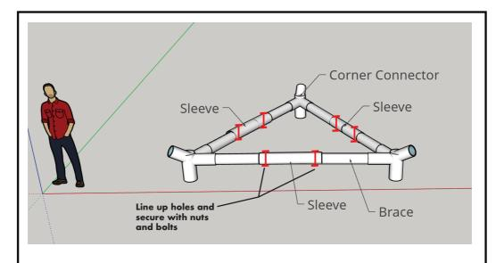
SLIDE SLEEVES SIDEWAYS TO COVER JOINT BETWEEN BRACING TUBES, LINE UP HOLES AND SECURE WITH NUTS AND BOLTS, AS SHOWN.
