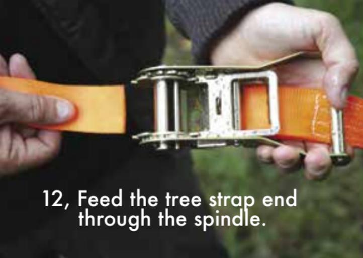
12, Feed the tree strap end through the spindle.
