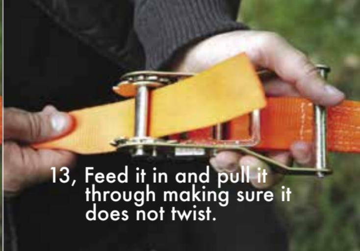
13, Feed it in and pull it through making sure it does not twist.
