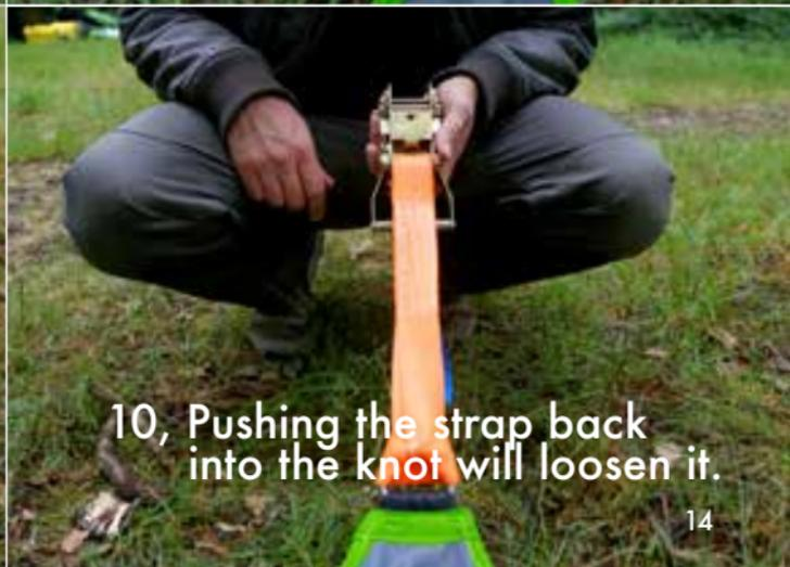
10, Pushing the strap back into the knot will loosen it.
