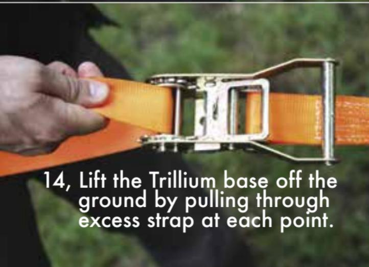
14, Lift the Trillium base off the ground by pulling through excess strap at each point.
