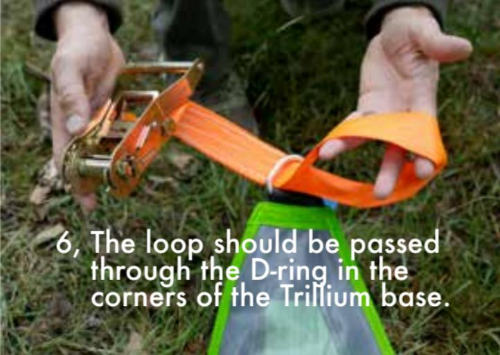
6, The loop should be passed through the D-ring in the corners of the Trillium base.
