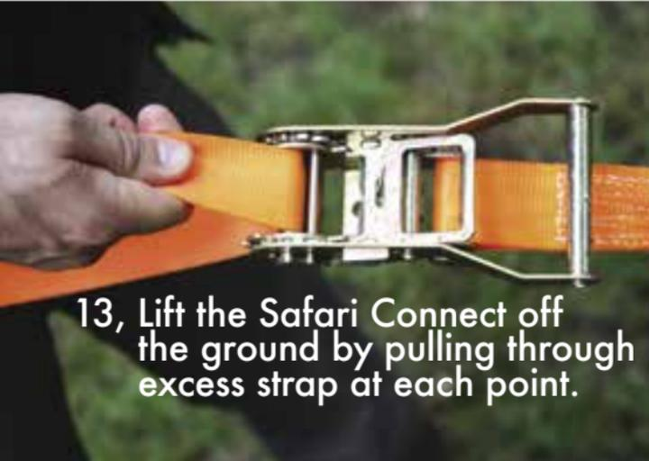
13, Lift the Safari Connect off the ground by pulling through excess strap at each point.
