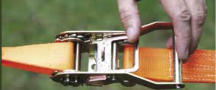
15, Release the ratchet lock by pushing the inner latch upwards.
