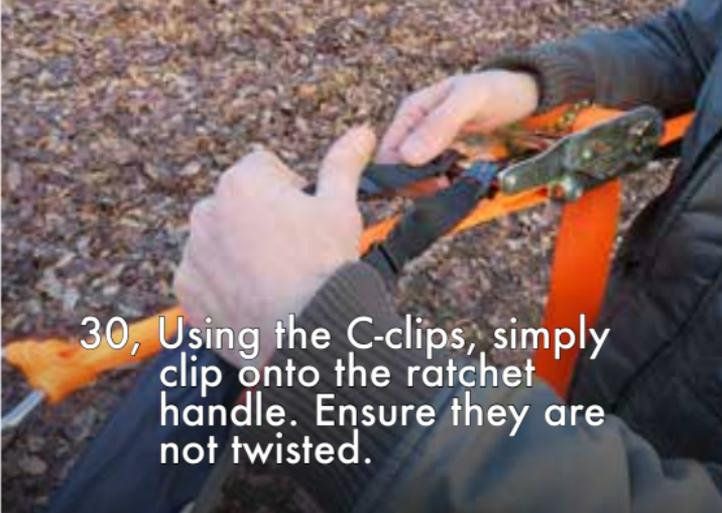
30, Using the C-clips, simply clip onto the ratchet handle. Ensure they are not twisted.
