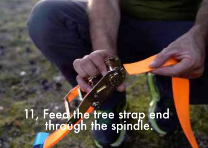
11, Feed the tree strap end through the spindle.
