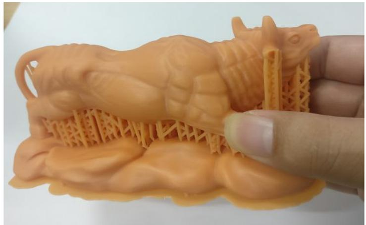
After your model is clean, put it in a cool, dry, well-ventilated area. To cure it, you may use a UV light machine or expose it directly to sunlight. After a few hours in the sun (or 20-30 minutes under a machine), the print will become fully dry and solid.
