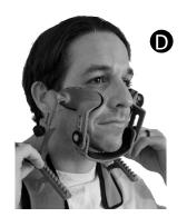
D) Turn both large knobs to retract head over shoulders. Count clicks to retract both sides evenly. Release cheek pressure by turning large knobs in the opposite direction. Release one post from track and open chin rest to remove collar when finished.
