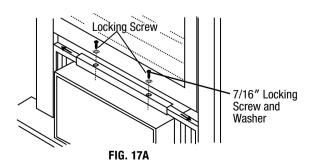
4. Attach the top angle to window frame: Use a 3/32" drill bit to drill one hole through the hole in the middle of top angle into the window frame, and drive one 3/4" (or 1/2") HEX-HEAD locking screw through hole in the middle of top angle into the window frame, as shown (Fig. 17B).
