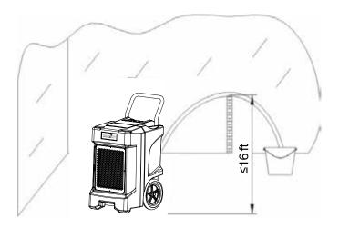
**NOTE:** The drain hose for the ejector pump is 40 ft long and can drain up to 16 ft vertically. Attempting to push water vertically more than 16 ft vertically may cause water backup in the pump, which can result in leakage. See image above.
