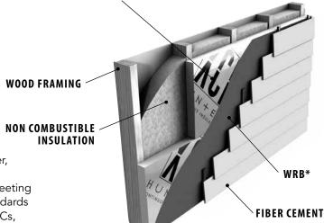
\* The location and number of WRB's in the wall assembly are determined by the architect.
