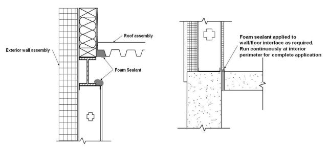
FIGURE 2—ROOF WALL JUNCTURE
