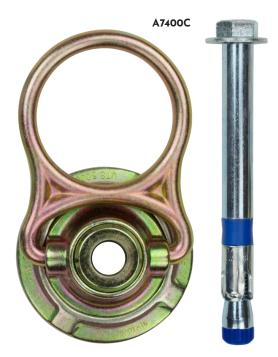
The10K Swivel Anchor (A7400) can be used on steel flanges while the A7400c is specifically designed for use in concrete. This particular anchor rotates 360 degrees and flips 180 degrees. The safe working load for this product is 2,000 lbs. with an ultimate breaking strength of 10,000 lbs. This anchor is composed of zinc plated steel.
