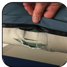
Torn Zipper Seam
