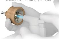
7. Remember the clue: tip to tip for perfect heat. Point the tip of the inner, blue jet flame to the tip of the golden heating chamber.
