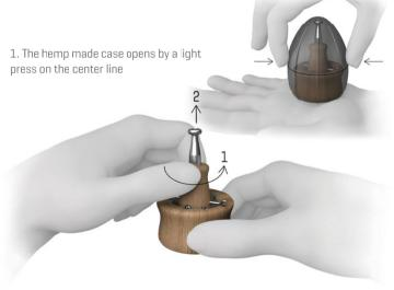
2. disassemble the upper part of vapman by twisting it counterclockwise
