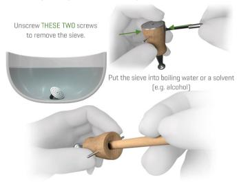
Take the backside of the cleaning brush to remove residues from the inside of the middle piece.
