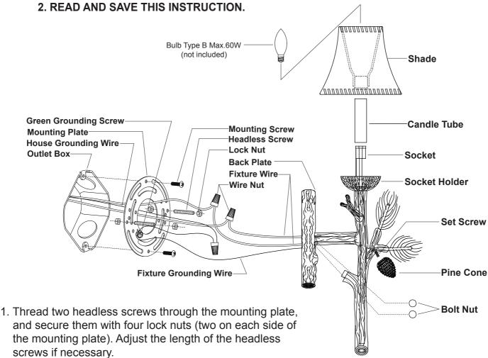
Note: Make sure that the headless screws are lined up horizontally, to ensure that the fixture will be level.
