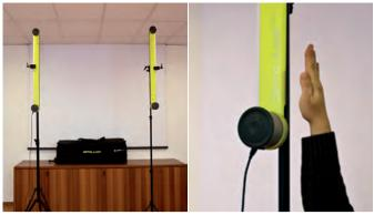
The OptoJump can duplicate the traditional vertical jump testing, and also provides a "Drift Protocol" to determine an athlete's dynamic stability.
