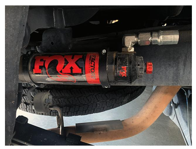
Figure 6: Installed reservoir
