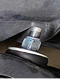
Figure 3: Rear lower eyelet installed
