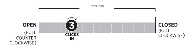
LEAST AMOUNT OF COMPRESSION DAMPING **SOFTEST**  GREATEST AMOUNT OF COMPRESSION DAMPING FIRMEST
