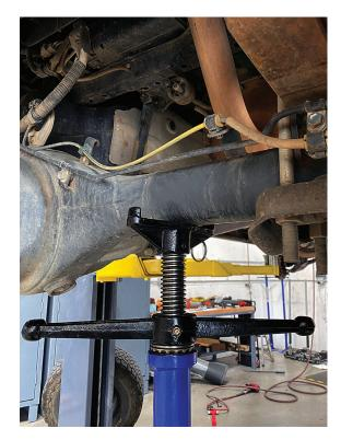
Figure 1: Axle jack supporting the axle
